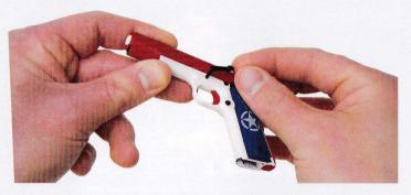
Drop Slide lock (B) into hole. Push slide back until it aligns with the small indent, set into place. Slide should easily move back and forth.
