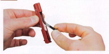
Insert pin (A) into spring (H). Push firmly into front bottom of slide. Hold spring down with finger to avoid popping out.
