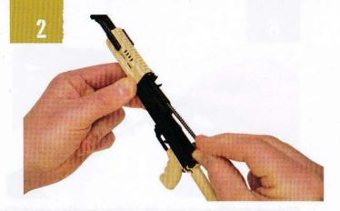
Slide spring cover bolt carrier. Front of bolt carrier inserts into charging handle. Rear sits in the channel.
