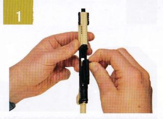
Insert charging handle with the flat end toward the barrel.
