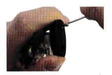
Place recoil pad insert at end of stock. Screw on recoil pad (I) using the 2 longest screws
