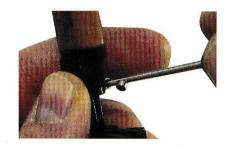
Slide barrel (A) onto upper receiver (B). Screw into place.
